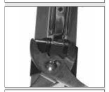
Fig. 7: Attach pin to tripod leg bracket with a large pliers (Style 2).
